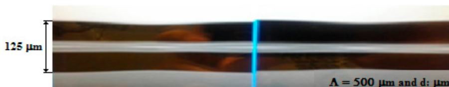
Figure 5. Microphotograph of the side view of the long-period grating sensor produced by arc discharges.
