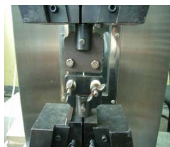
Figure 12 Electronic universal testing machine for measuring the length and diameter of each optic nerve specimen.
