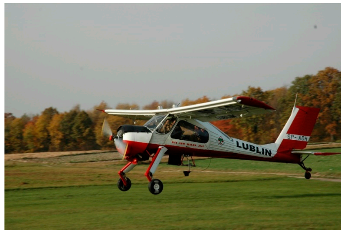
Figure 4. The airplane used for the flight tests: the PZL 104 Wilga with the CORREVIT optical sensor.
