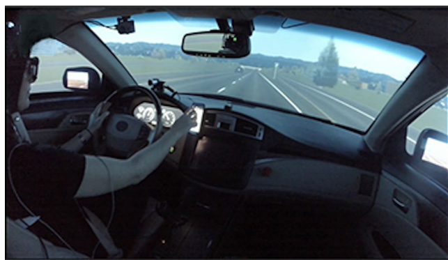
Figure 3. In-cabin view of the driver and their surroundings. Participant's experienced a 270° field of view of the driving environment, including rear projection for the rear-view mirror and LCD-screen side mirrors. The smartphone was attached to a standard aftermarket magnetic dash mount.
