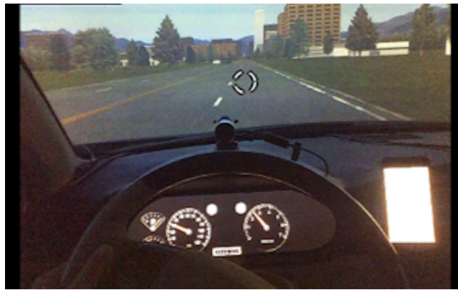
Figure 5. Single frame image from a participant's eye-tracking video. The analysis software superimposed a fixation point (i.e., white circle on the road in this image) onto each video frame. For each frame the location of the participants fixation was manually coded as being on the road, phone, cab, or outside of the cab in a location other than the road. In the current image, the location would be coded as "road". Coding of the videos in this manner allowed us to calculate the total duration viewed for each region, as well as viewing patterns during each of the distracting events.
