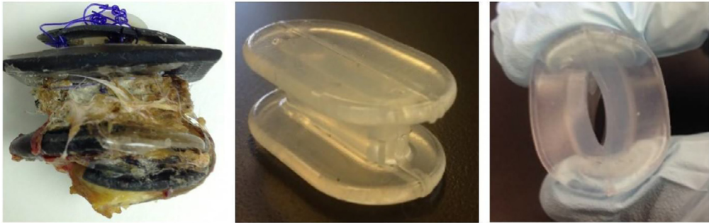
1. Previous design after removal from animal, showing evidence of significant rejection. 2. Final design of silicone port, produced with 3D printing and molding techniques. 3. Final design of port, showing slit allowing for endoscopic access.
