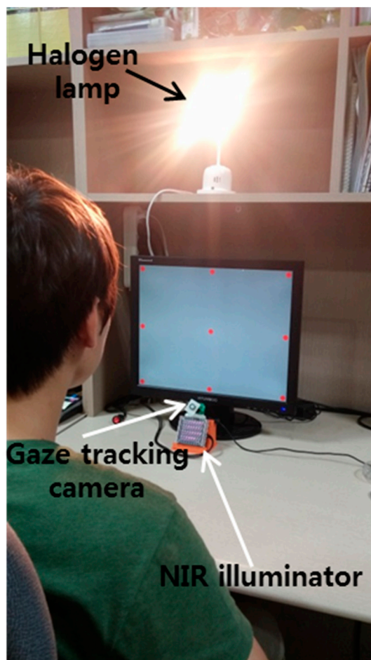
Figure 19. Experimental setup for measuring gaze tracking accuracy under a halogen lamp.
