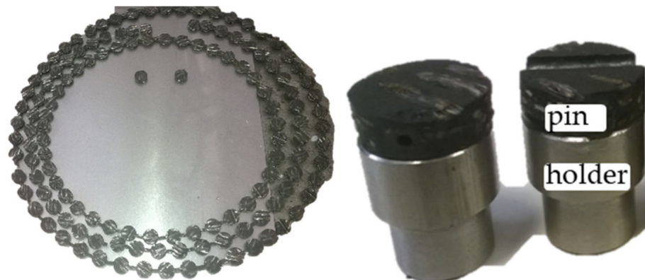
Figure 3. Samples cut from the facing and glued to metal holder-pins for fixation.
