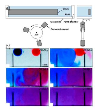
**Figure 3.** The experimental setup and results of [103] for individually controlling two cilia in a fluid chamber. (a) The setup configuration and (b) time lapse images with the best performed alternate pattern cilia beat. Reproduced with permission from [103], published by the ASME, 2017.
