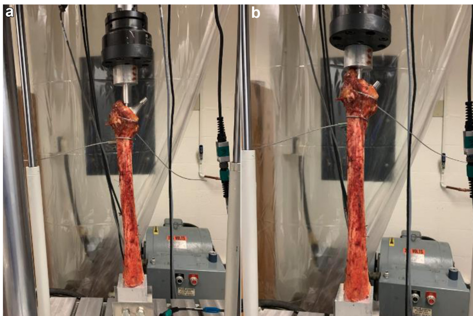
Figure 5. (a) Cadaveric femur with cables after periprosthetic fracture. (b) Cabled cadaveric femur retested on an MTS machine after fracture.
