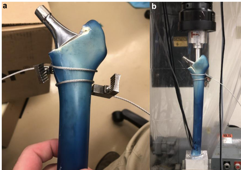
Figure 7. (a) Composite Sawbone femur with cables after an initial fracture. (b) Periprosthetic fracture created during biomechanical testing after cabling.
