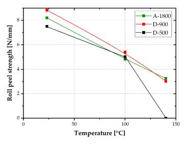
**Figure 8.** Roll peel strength at 23, 100 and 140 °C of laminates made from epoxy varnishes with EEW values of 500, 900 and 1800 g/mol.
