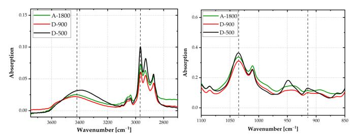
**Figure 4.** FTIR-ATR spectra in the range from 3700 to 2700 cm<sup>-1</sup> (**left**) and 1100 to 850 cm<sup>-1</sup> (**right**) of epoxies with average EEW values of 500, 900, and 1800 g/mol.
