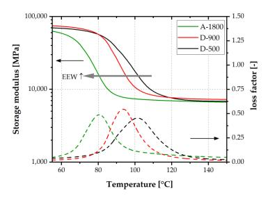
**Figure 7.** Storage modulus and loss factor curves of electrical steel laminates adhesively bonded with epoxy varnishes with EEW values of 500, 900 and 1800 g/mol.
