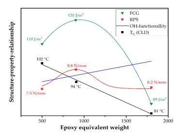
**Figure 10.** Schematic relationship of OH functionality, crosslinking density (CLD), roll peel strength (RPS) and fatigue crack growth kinetics (FCG) at ambient temperature and the epoxy equivalent weight (EEW) of the adhesive in electrical steel laminates.
