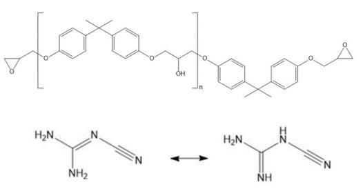
**Figure 1.** Chemical structure of DGEBA with repeating unit n (**top**) and DICY (**bottom**) with its two tautomeric forms, diamino (**left**) and amino-imino (**right**).
