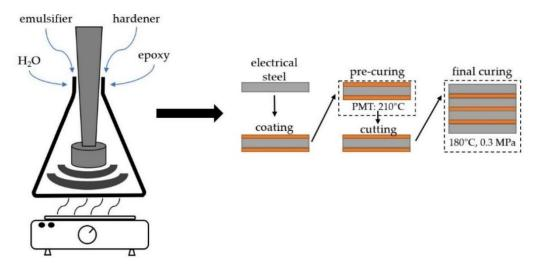
**Figure 2.** Schematic illustration of varnish preparation (**left**) and electrical steel coating, stacking and lamination (**right**).
