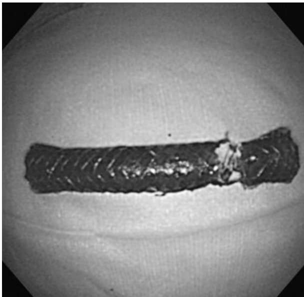
Fig. 4. A whole feature of fractured self-expandable metal stent was shown after endoscopic retrieval of the stent.
