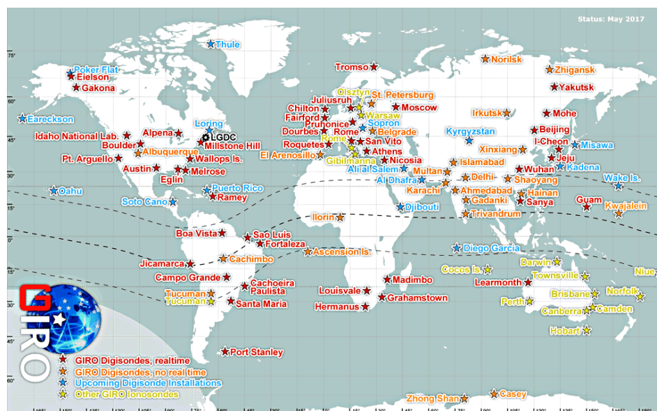
Figure 2. Map of digisondes contributing data to the Global Ionospheric Radio Observatory (GIRO). Red stars identify online digisondes providing data to GIRO in near-real-time, orange stars denote digisondes providing data to GIRO in no real time, yellow stars denote other type of ionosondes that also contribute to GIRO archives, and blue stars correspond to digisonde installations planned for the next future.
