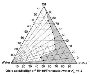
Figure I Pseudo-ternary phase diagrams of microemulsion systems under  $K_m = 1:2$ .
