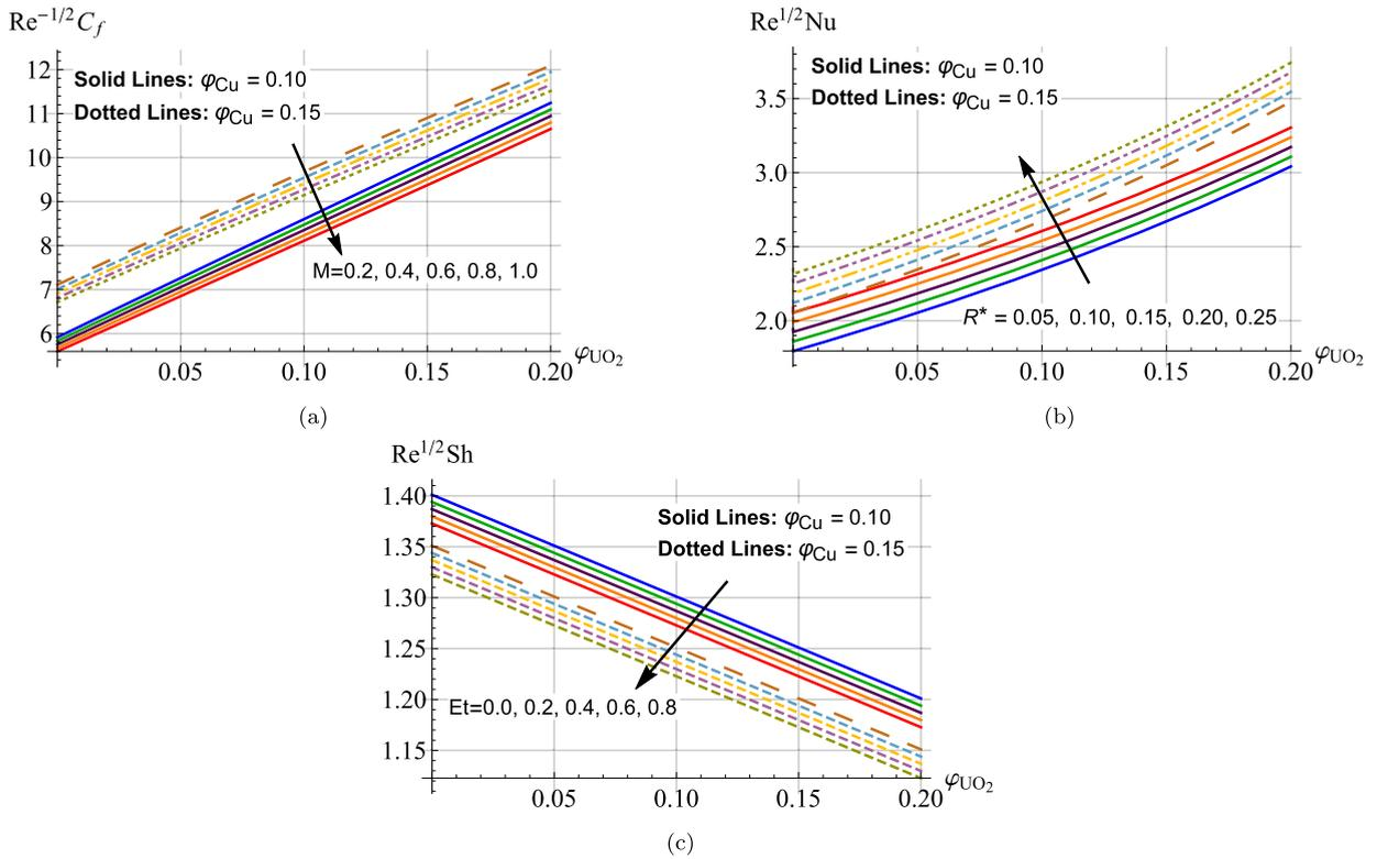
Fig. 6. Skin friction, heat transfer and mass transfer for different volume fractions of Cu.
