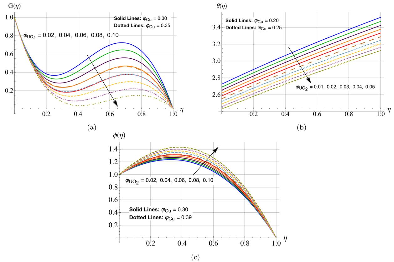
Fig. 5. Tangential velocity, temperature and concentration for different volume fractions of Cu.
