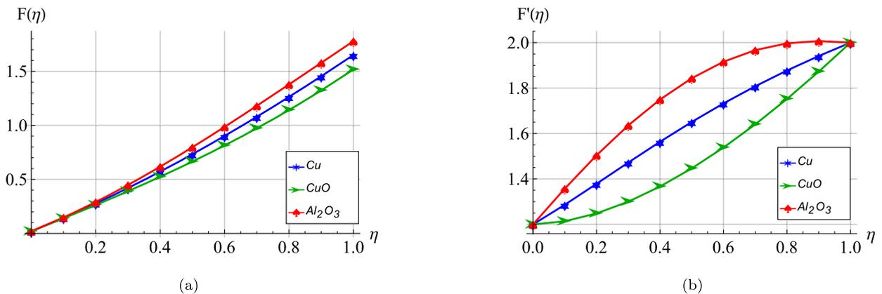
Fig. 7. Axial and radial velocity for different nanoparticles.
