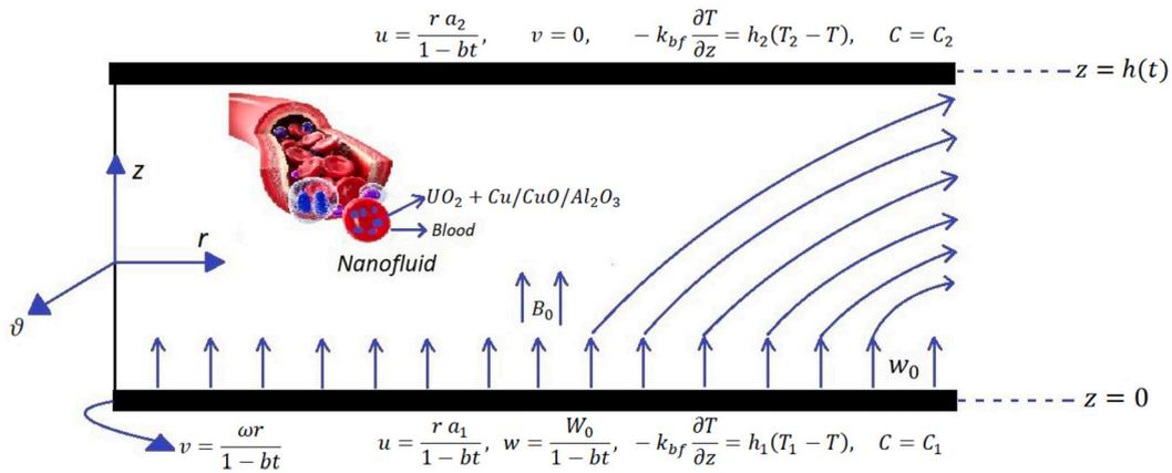
Fig. 1. Blood flow geometry.
