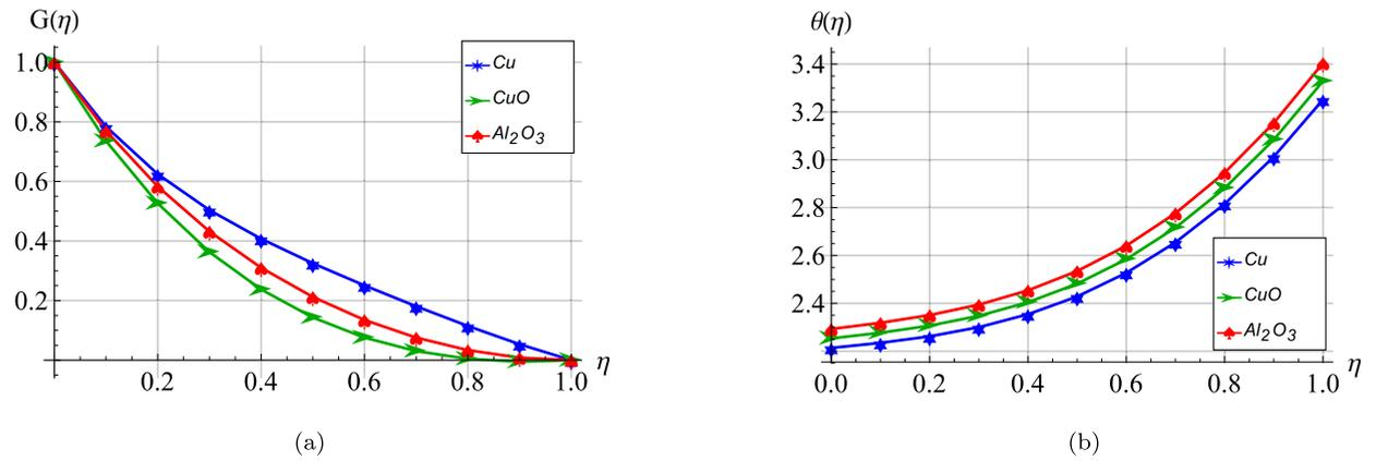
Fig. 8. Tangential velocity and temperature for different nanoparticles.
