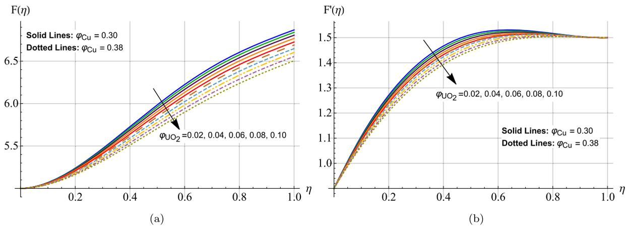
Fig. 4. Axial and radial velocity for different volume fractions of Cu.
