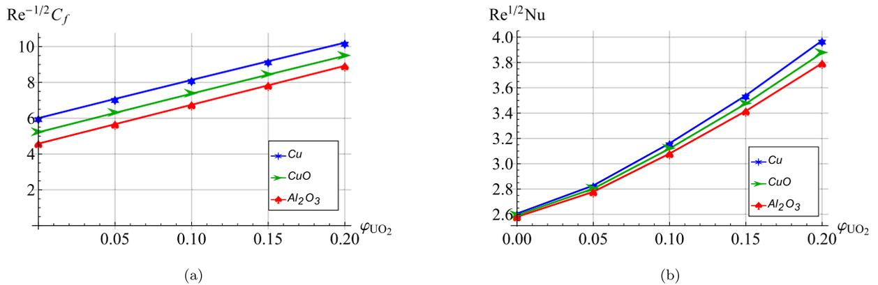
Fig. 9. Skin friction and Nusselt number for different nanoparticles.
