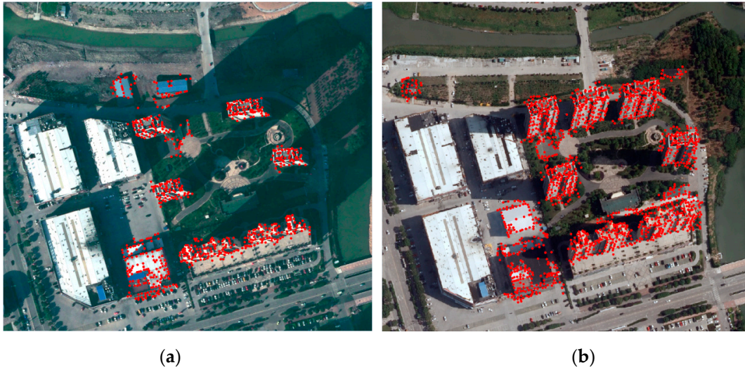
Figure 7. Feature detection. (a) Feature points detected in building change proposals at times t_1 and (b) t_2 .
