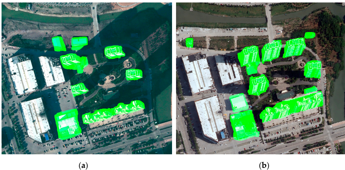
Figure 6. Changed building proposals in the bi-temporal aerial images at (a) time t_1 and (b) at time t_2 .
