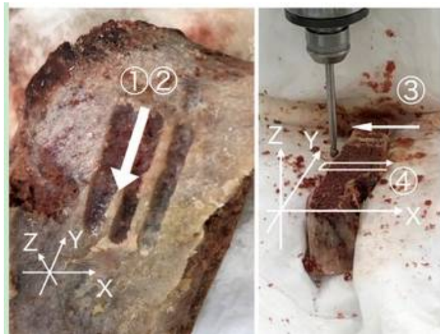
Figure 1. Relationship between the material and the grinding procedure. The left figure is a photograph after manual grinding of the cortex. The photo on the right is the machine procedure. Every series was repeated three times and recorded in the data logger.
