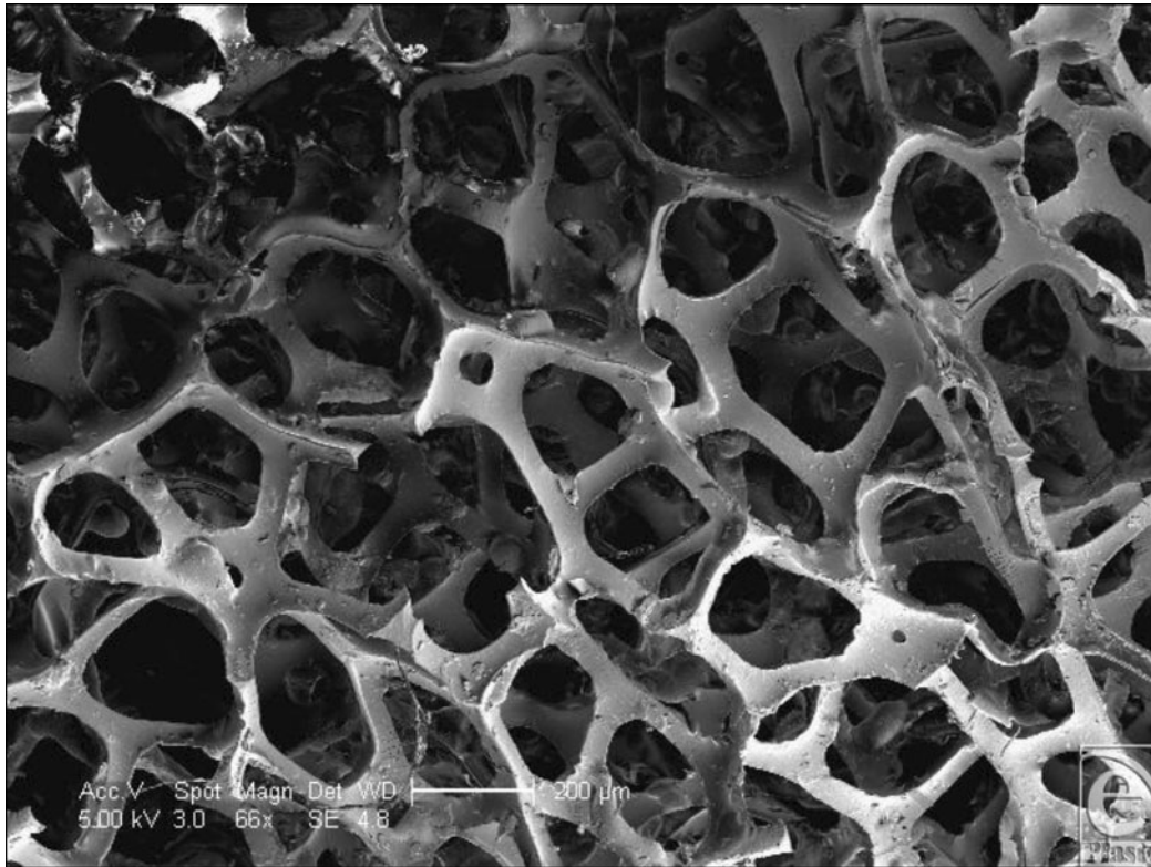
Figure 13. Polytech MicroPolyurethane Polyurethane (Polytech Silimed Europe GmbH) surface in scanning electron microscopy at 66\times magnification with a 200\text{-}\mu\text{m} scale bar. This image shows the fibrillar nature of the polytech polyurethane surface at high magnification. The cut ends of the polyurethane foam, where it is trimmed during manufacture and the network of fibrils is evident at this magnification. These fibrils are less circular in cross section than one might expect at lower magnification and each fiber is seen to have a sharp-bordered structure to it.
