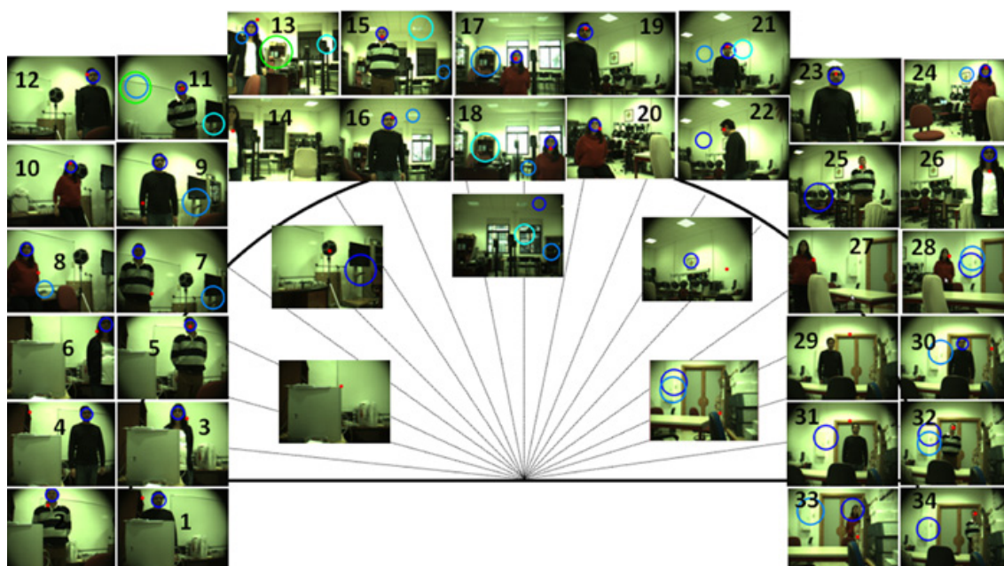
Figure 6. Visual localization system performance compared to a face-detector algorithm in five different backgrounds displayed in the images placed inside the circumference. The red circle on the image represents the visual system estimation. Blue circumferences show OpenCV face-detector estimations.
