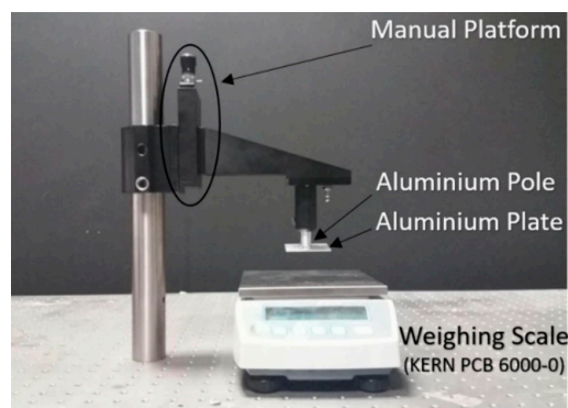
Figure 3. Set up for loading pressure.
