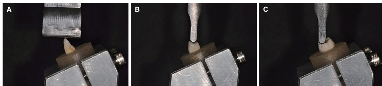
Fig. 1. (A) Fixtures employed for compression loading on incisor teeth, (B) Fixtures employed for compression loading on premolar teeth, (C) Fixtures employed for compression loading on molar teeth.
