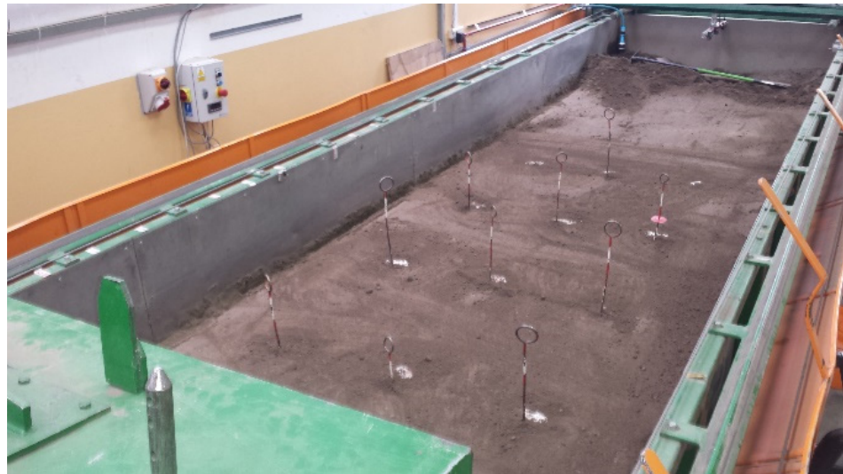
Figure 2. Compacted soil with stones embedded in three rows at a distance of 0.33 m and five columns at a distance of 0.80 m to the trials with coulters, whose edge was set in the axis of the stones row impacting the stones in the middle of their length.
