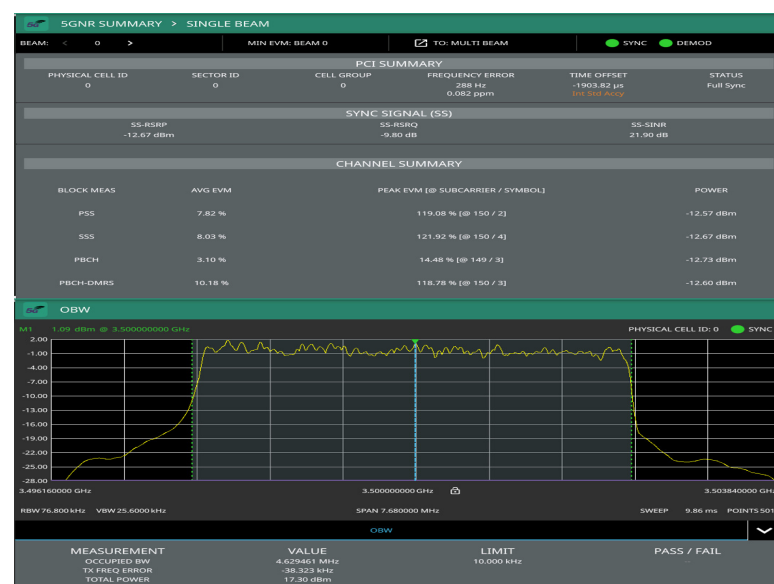
Figure 4. Transmitted signal demodulation, occupied bandwidth, channel power, and spectrum from the implemented gnodeB.
