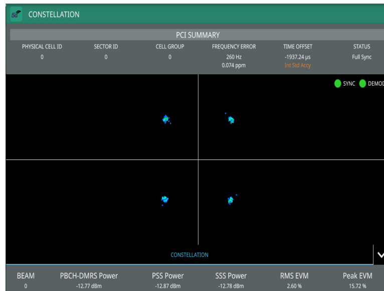
Figure 5. Q-PSK modulation scheme representation of the PBCH in the gnodeB measured through the MS2090A-Anritsu.
