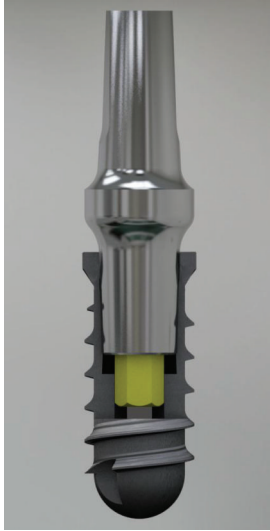
FIGURE 14: The implant used in this report is characterized by a cone Morse taper interference-fit (TIF) locking-taper combined with an internal hexagon. The Morse taper presents a taper angle of 1.5°.
