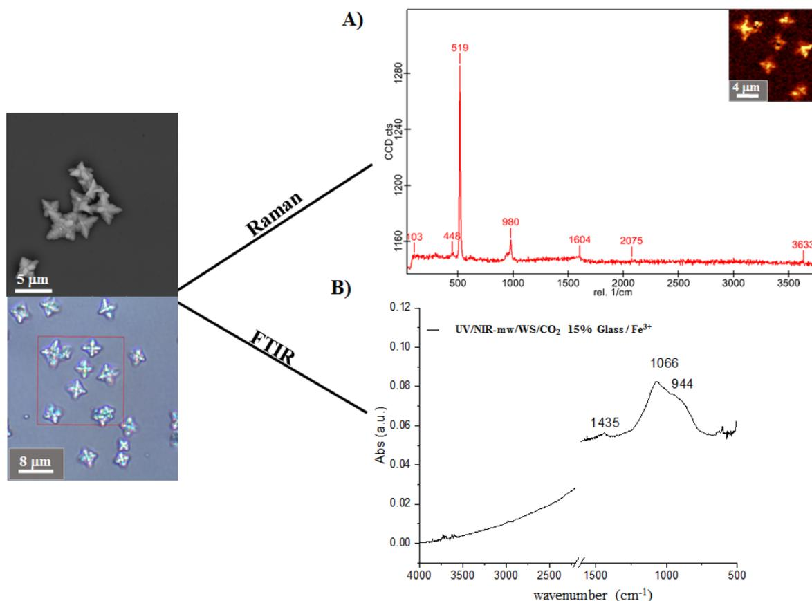
**Figure 6.** Representative image of the biomorphs obtained in the presence of  $\text{Fe}^{3+}$  (SEM, optical, and confocal images), in the four analyzed atmospheric conditions: STP, UV/NIR-mw/ $\text{CO}_2$ atm, UV/NIR-mw/WS/ $\text{CO}_2$  atm, or UV/NIR-mw/ $\text{CO}_2$  15%. Identification of the crystalline phase of biomorphs through (A) Raman and (B) FTIR spectroscopy.
