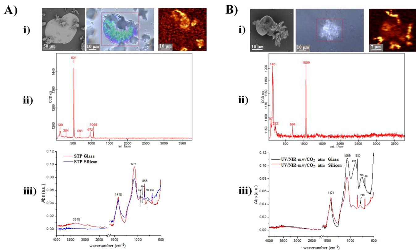
**Figure 2.** Identification of the crystalline base of the BaCO<sub>3</sub> biomorphs through Raman spectroscopy and FTIR. (A) Control sample. (B) Sample synthesized with UV light. (i) SEM, optical, and confocal images. (ii) Raman spectra. (iii) FTIR spectra. The BaCO<sub>3</sub> biomorphs show a witherite crystalline structure.
