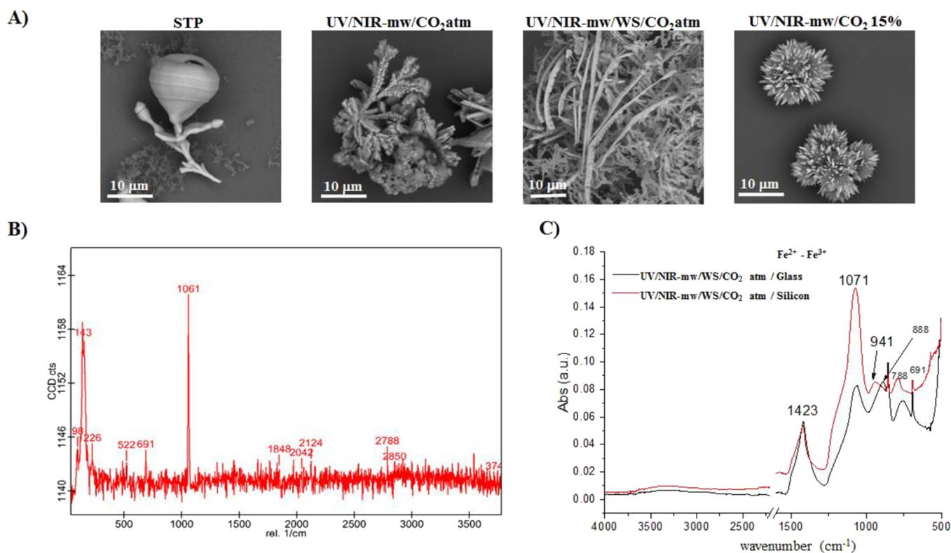
**Figure 7.** Representative images of the biomorphs obtained in the presence of the  $\text{Fe}^{2+}/\text{Fe}^{3+}$  mixture with the four analyzed atmospheric conditions: STP, UV/NIR-mw/ $\text{CO}_2$ atm, UV/NIR-mw/WS/ $\text{CO}_2$ atm or UV/NIR-mw/ $\text{CO}_2$  15%. (A) Identification of the crystalline phase of biomorphs by (B) Raman and (C) FTIR spectroscopy.
