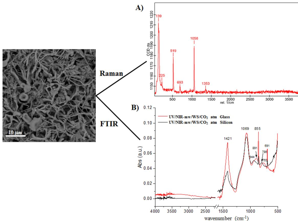
**Figure 4.** Analysis of biomorphs synthesized under UV/NIR-mw/WS/CO<sub>2</sub> atmosphere. Identification of the crystalline phase of the biomorphs by (A) Raman and (B) FTIR spectroscopy.
