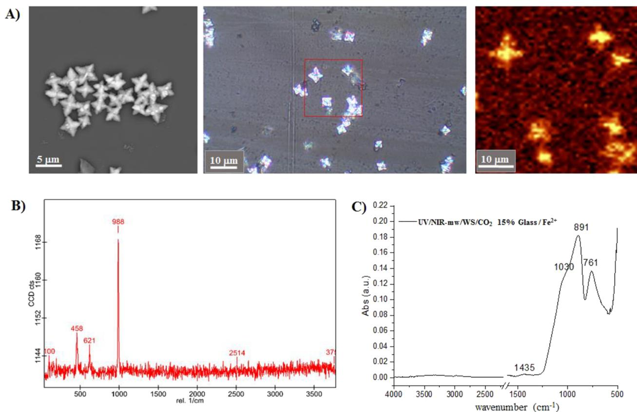
**Figure 5.** Representative image of the biomorphs obtained in the presence of  $\text{Fe}^{2+}$  in the four atmospheric conditions analyzed in this study: STP, UV/NIR-mw/ $\text{CO}_2$ atm, UV/NIR-mw/WS/ $\text{CO}_2$ atm, or UV/NIR-mw/ $\text{CO}_2$  15%. (A) SEM, optical, and confocal images. (B, C) Identification of the crystalline phase of the biomorphs through (B) Raman and (C) FTIR spectroscopy.
