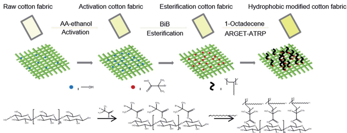
Fig. 2 Schematic of preparation of hydrophobically modified cotton fabric.
