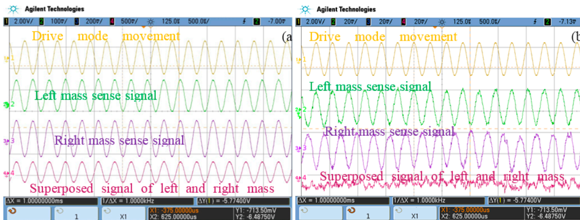
Figure 4. (a) Test signals before quadrature error correction; (b) Test signals after quadrature error correction using the correction method with the two masses together.
