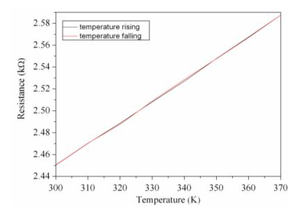
Figure 9. Resistance of the generator.
