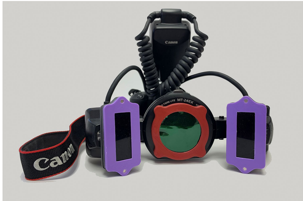
Fig. 1 Camera set up used for the study. Violet colored plastic indicates the UV filters on flash lamps and red plastic the green filter on the lens
