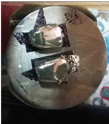
Figure 1: Gold coating of the tooth surface for the scanning electron microscope analysis
