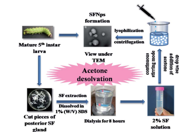
Fig. 1 Scheme representing fabrication of AA-SFNps from matured 5 th instar larvae using acetone desolvation procedure.
