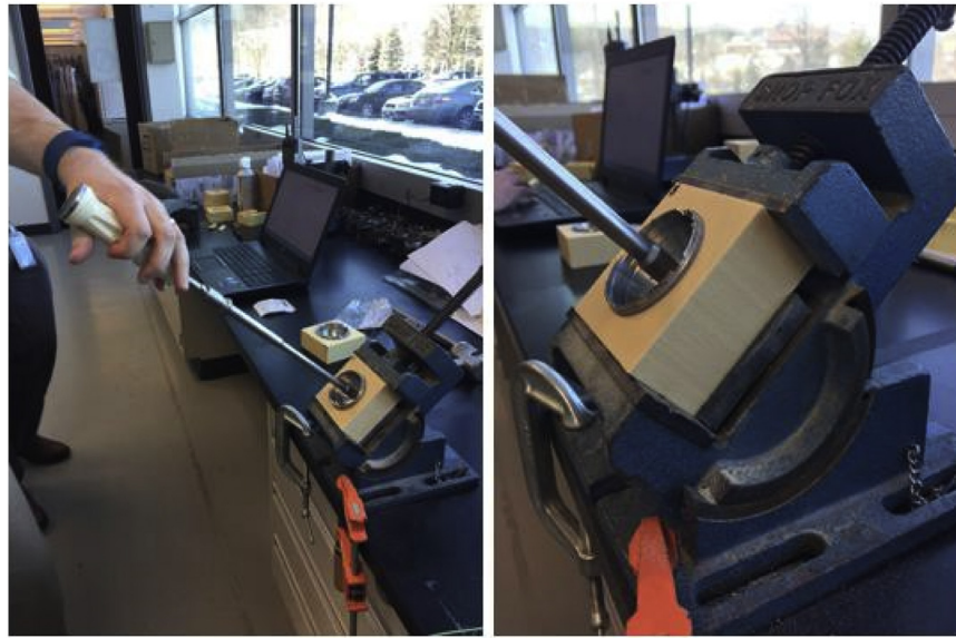
Figure 3. Experimental setup with instrumented mallet and force sensor impacting an acetabular component into a premachined Sawbones cavity.
