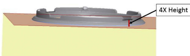
Figure 4. Seating height measurement.
