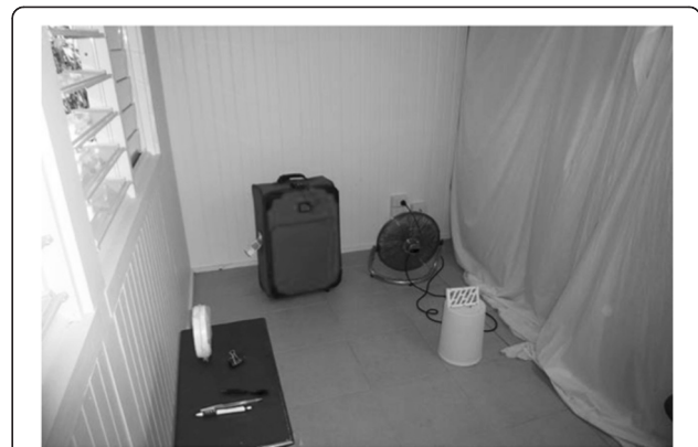
Figure 1 Experimental room 3. Room used in open room trials showing a suitcase, metofluthrin emanator (on bucket), open louvered window and Clark sentinel ring on table. The small table fan was turned on low and faced away from the emanator, generating wind speed of 0.2 m/s at the emanator located 1 m way.
