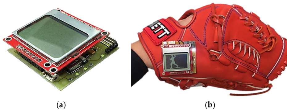
Figure 4. Display device of wearable assist system (a) LCD display device, (b) the device attached to the baseball glove.
