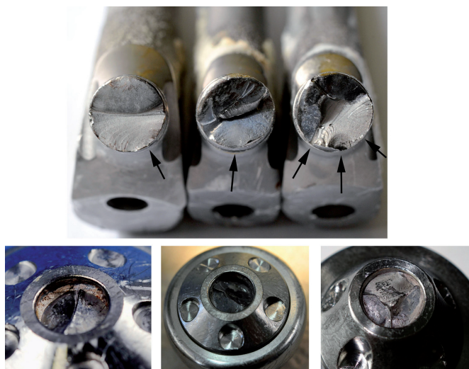
Figure 3. Upper panel: Stem fracture surface with fatigue cracks radiating out from the origin of the crack (black arrows) as a series of concentric rings (rest lines; left to right: cases 1 to 3). Case 3 had 3 crack origins, which subsequently coalesced into a unified fracture.
