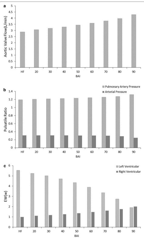
**Fig. 5** The mean flow of aortic valve, pulsatile ratio and external work. **a** The mean flow of aortic valve with support level (BAI) of LVAD; **b** PR of pulmonary artery pressure and arterial pressure with support level (BAI); **c**: EW of left ventricular and right ventricular with support level (BAI)
