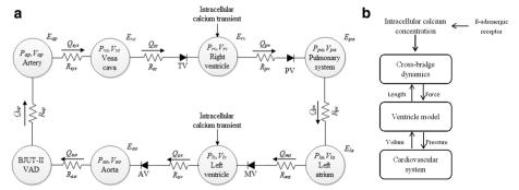
**Fig. 1** Schematic of multi-scale model. **a** Multi-scale lumped parameters model; **b** schematic of the interconnect model of the cardiovascular system
