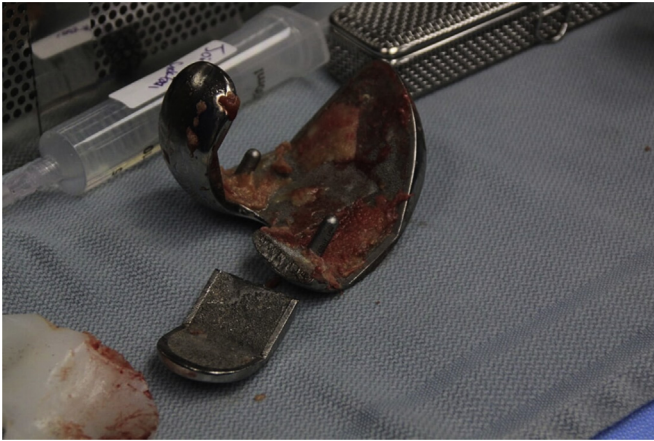
Figure 4. Intraoperative photograph displaying the fractured medial component of the Medial-Pivot Knee System once the prosthesis was fully extracted.
