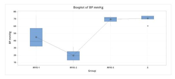
**Figure 7.** Boxplot of BP test. Mean maximum BP values for each group in Study arm 1. Group S, Stapler; Group RFVS-1, LigaSure 5 mm Dolphin tip; Group RFVS-2, ENSEAL; Group RFVS-3, LigaSure Atlas 10 mm; BP, Burst Pressure). Group HS was not tested because of sealing failure in all samples. RFVS-1 was significantly lower (p < 0.05) than the RFVS-3 and S groups, but significantly higher than the group RFVS-2, which recorded the significantly lowest values (p < 0.05). \*: outlier.
