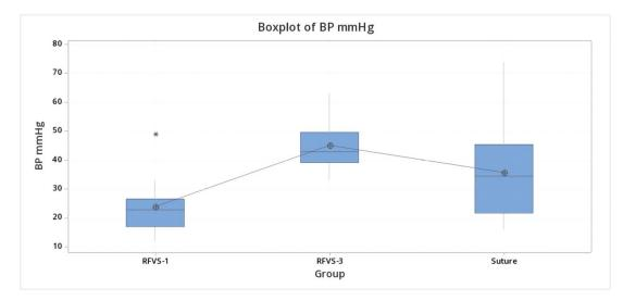
**Figure 10.** Boxplot of BP test. Mean maximum BP values for each group in Study arm 1. Group Suture; Group RFVS-1, LigaSure 5 mm Dolphin tip; Group RFVS-3, LigaSure Atlas 10 mm; BP, burst pressure). The group RFVS-1 resulted in significantly lower BP values (p < 0.05). Otherwise, RFVS-3 and the Suture group showed comparable BP pressures (p > 0.05). \*: Outlier.
