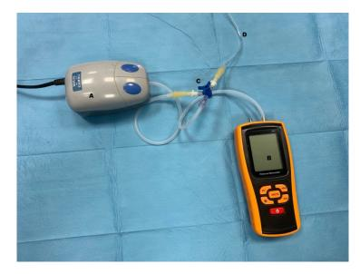
**Figure 3.** Image of instrumentation used for burst pressure (BP) test. (**A**) air pump; (**B**) manometer; (**C**) three-way stopcock; (**D**) tube to the construct.
