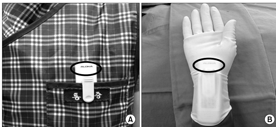
Fig. 1. Two dosimeters were used to record the radiation exposure. (A) One was worn on the left chest over the lead apron. (B) The other was worn on the palmar aspect of the right hand. Circle: detector of dosimeter.
