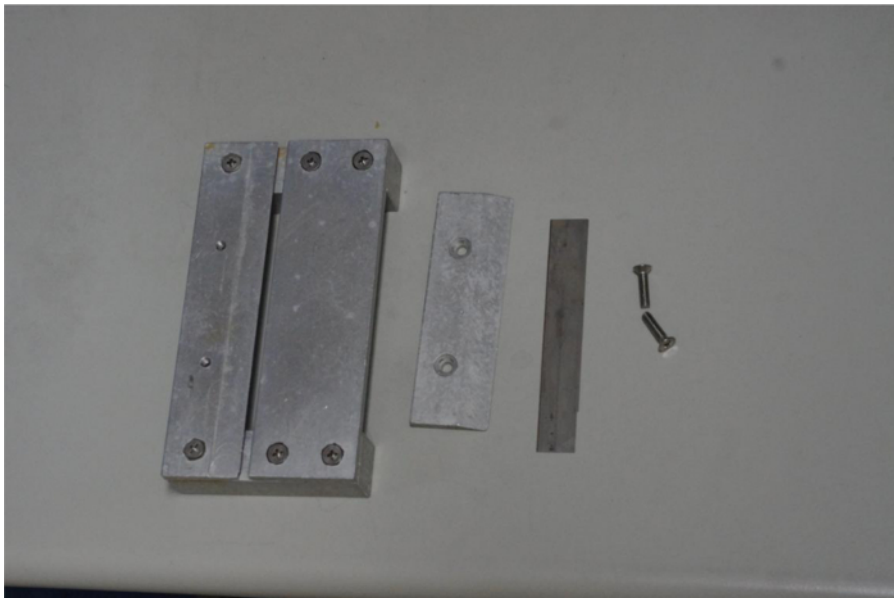
Figure 1. A customized slicer used for isolation of pADSC. Dissected adipose tissues from porcine dorsal subcutaneous adipose tissues are composed of the fat layer with attached skin layers. A slicer is required to slice the fat layer approximately 1 mm thick with avoidance of over-slicing into the skin layers. From left to right: slice holder, slicer pad, carbon steel slicer blade, and screws. Slicer blade is inserted between slice holder and slicer pad when assembled. Please click here to view a larger version of this figure.
