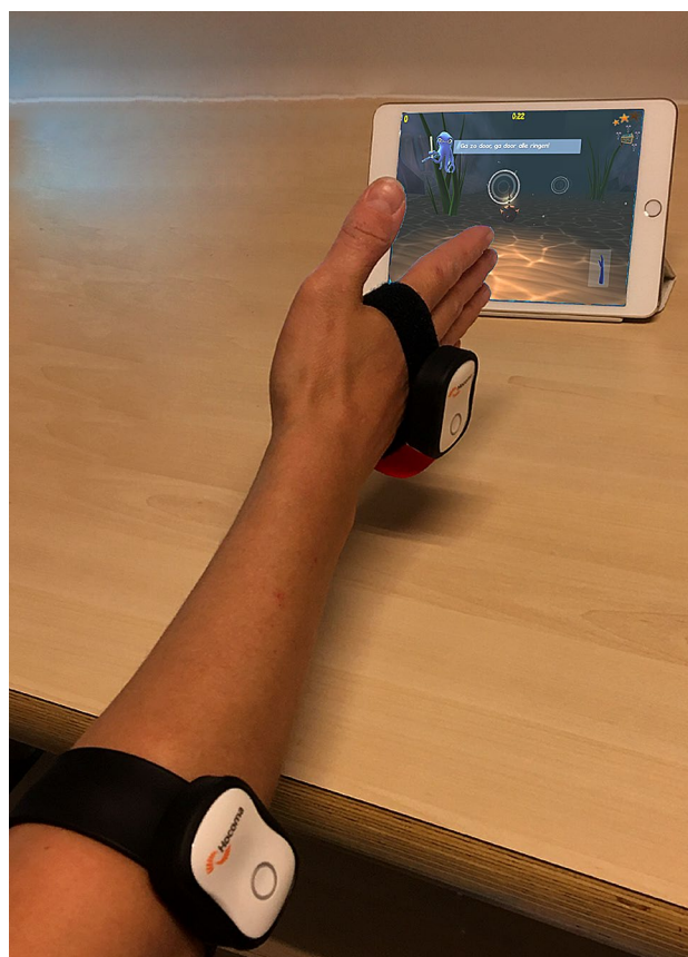
Fig. 1 Setup of the Valedo® sensors around dorsum of the hand and lateral side of proximal forearm
