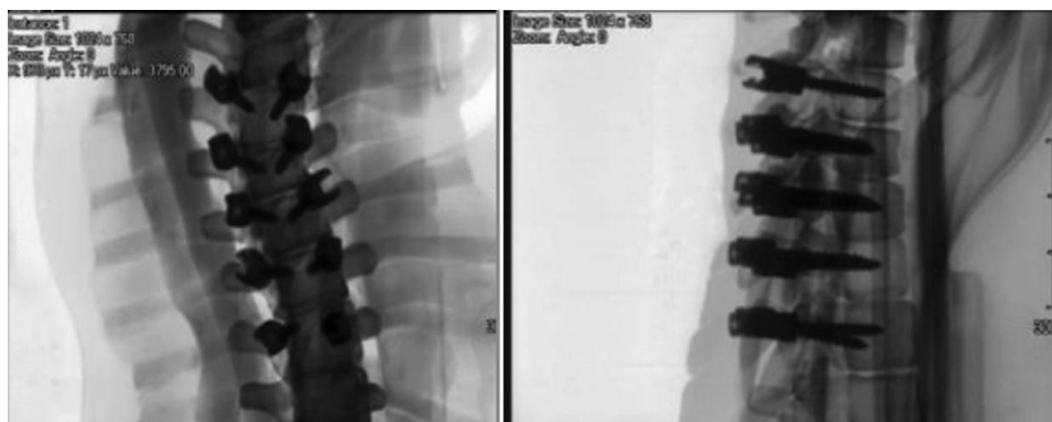
Figure 2. AP and lateral radiographic view of sawbones post instrumentation.
