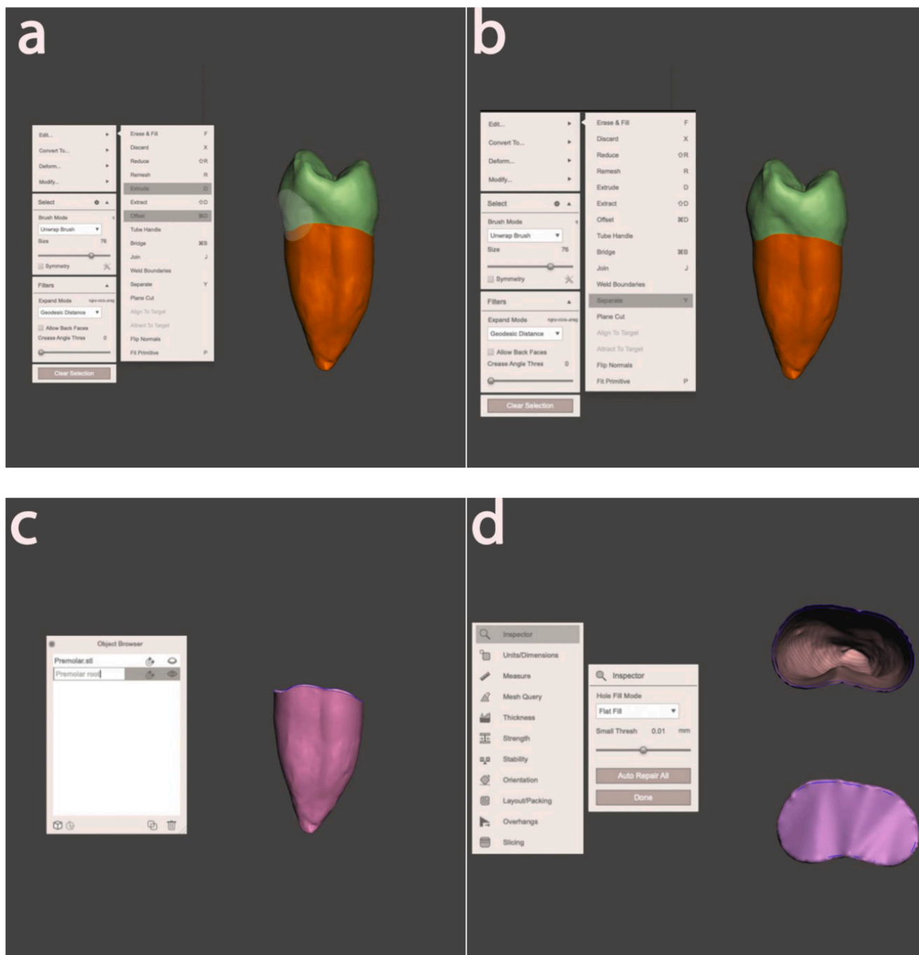
Fig. 3. The design process with a non-dental open-source software program. a, Software view of the tooth crown separate from the root surface. b, Software view of the original file for the separate root shell according to the tooth name. c, Software view of the outline of making a duplicate root surface. d, Software view of the outline of the filled root surface.
