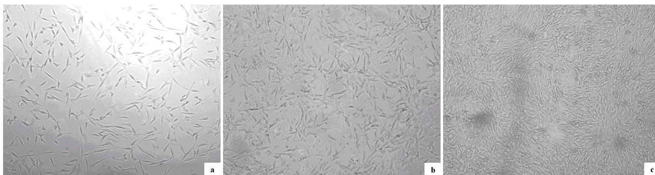
Figure 7. Optical micrographs (100×) of 3T3 fibroblasts cultured on (a) glass as control; (b) PLA; and (c) collagen-PLA.
