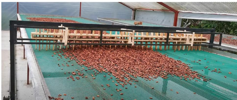
**Figure 4.** Removal module of the automated removal prototype for the natural drying of the cacao bean.
