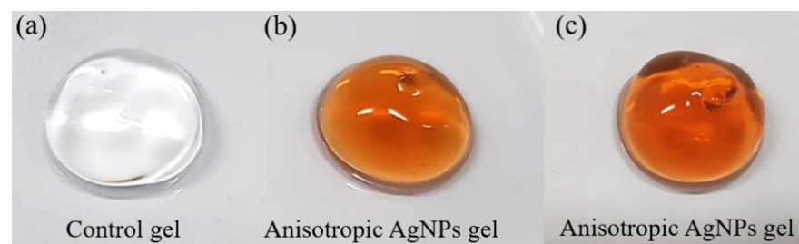
Figure 1. Anisotropic AgNPs containing formulation. Gel without AgNPs (a), Gel containing 0.04 mg/g of anisotropic AgNPs stored at room temperature (27–30 °C) for 24 h (b) and 1 year (c).
