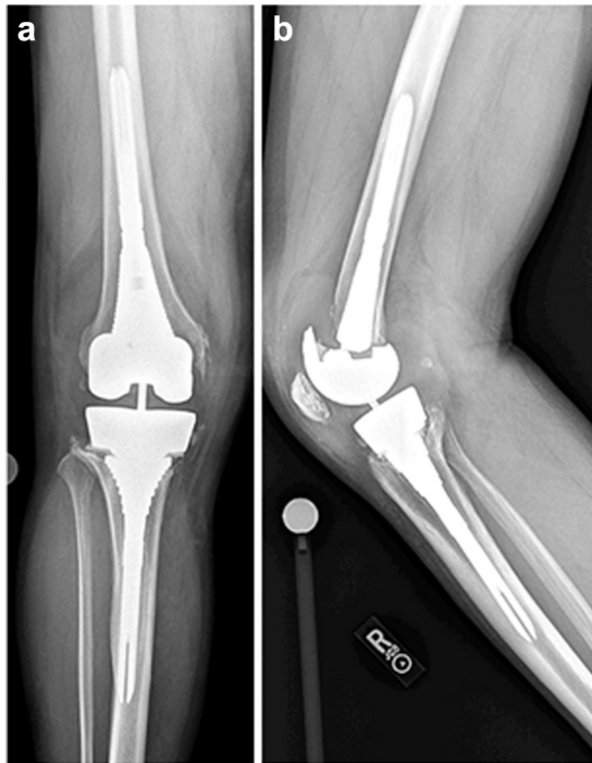
Figure 2. Anteroposterior (a) and lateral (b) views obtained 3 years after revision confirmed fracture of the implant at the adapter. Again, there is disruption of the 90° relationship between the adapter and the femoral component on the lateral view.
