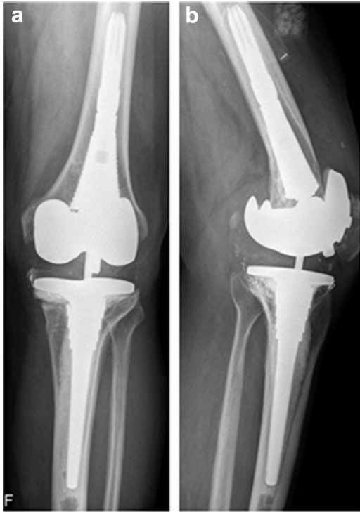
Figure 4. Anteroposterior (a) and lateral (b) views obtained 6 years after revision confirmed fracture of the implant at the adapter bolt. The fractured bolt is seen in the joint space on both views.
