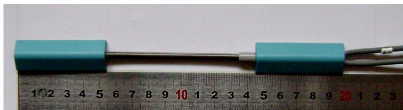
Figure 3. The biaxial goniometer (Biometrics Ltd., Gwent, UK; blue model [XM110]), used for knee recordings.
