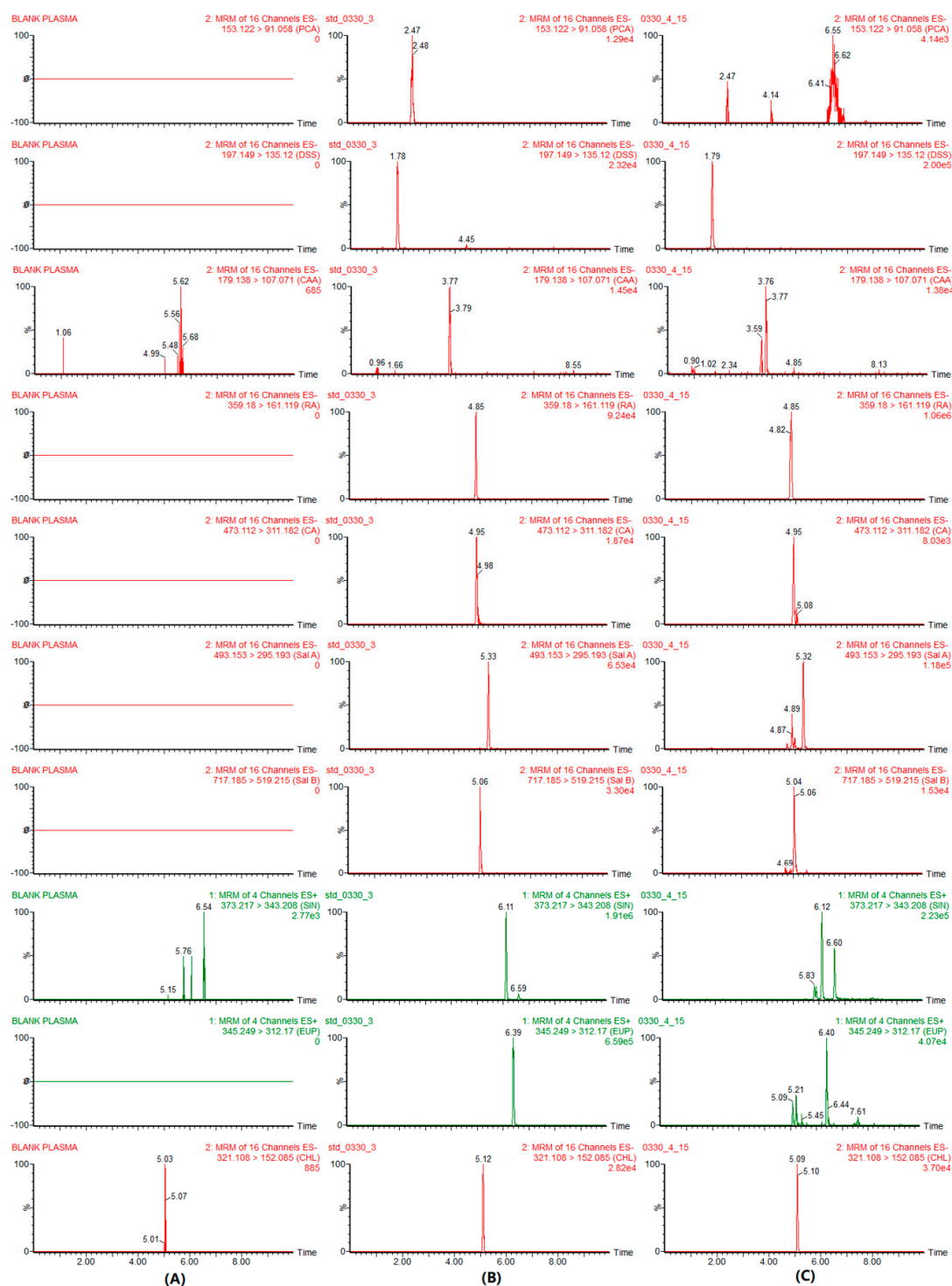
Figure 1. Typical multiple reaction monitoring (MRM) chromatograms of blank plasma (A); blank plasma spiked with the nine analytes and IS (B); a representative plasma sample at 15 min after oral administration of the Orthosiphon stamineus Benth. (OS) extract (C).
