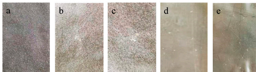
Figure 2. Films of SPI and fractionated products: (a) SPI, (b) lower protein, (c) upper protein, (d) 11S globulin, and (e) 7S globulin.
