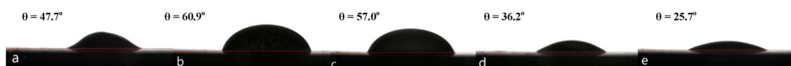
Figure 4. Contact angle of the film solutions of SPI and fractioned products: (a) SPI, (b) upper protein, (c) lower protein, (d) 11S globulin, and (e) 7S globulin.
