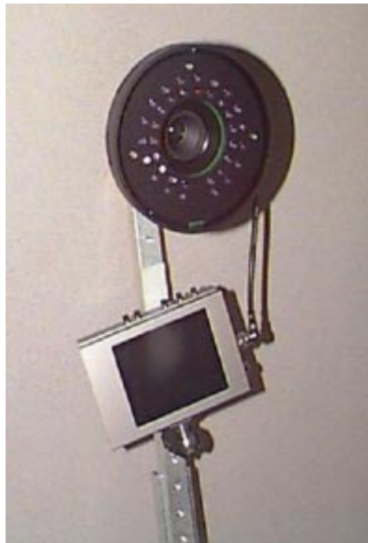
FIG. 1. The IR source and CCD detector that constitute the Varian RPM™ system
